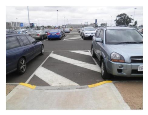
Figure 6 – Pedestrian path not clearly defined and poor sight lines
